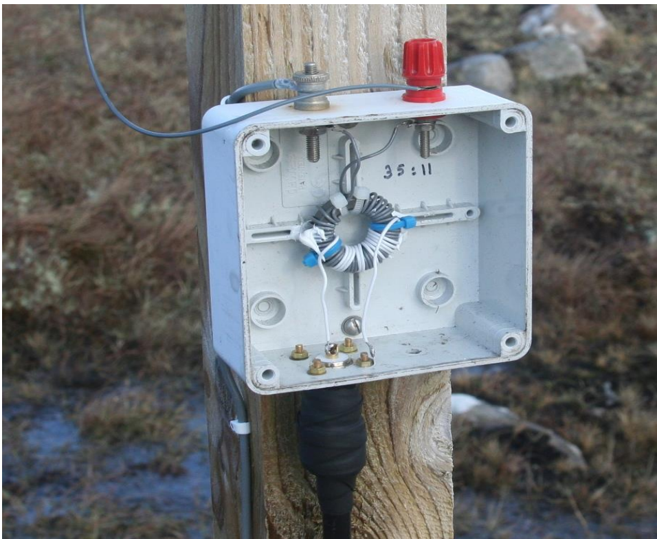
Fig 9: Transformer Box Mounted on Post with Close-up Showing Construction Detail
