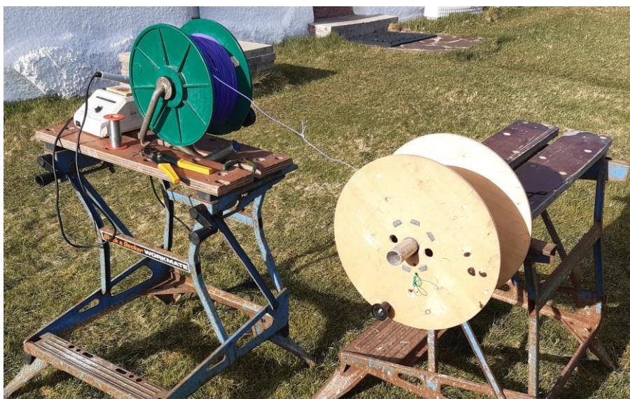
Fig 16: Arrangement for Checking and Refurbishing the Wire
